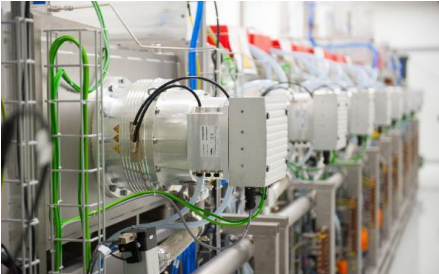
Application of metal layer in low pressure (DC Magnetron-sputtering)
